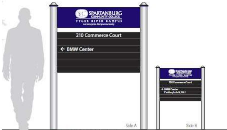
Sign Type A4 / Vehicular Directional Location V.11
