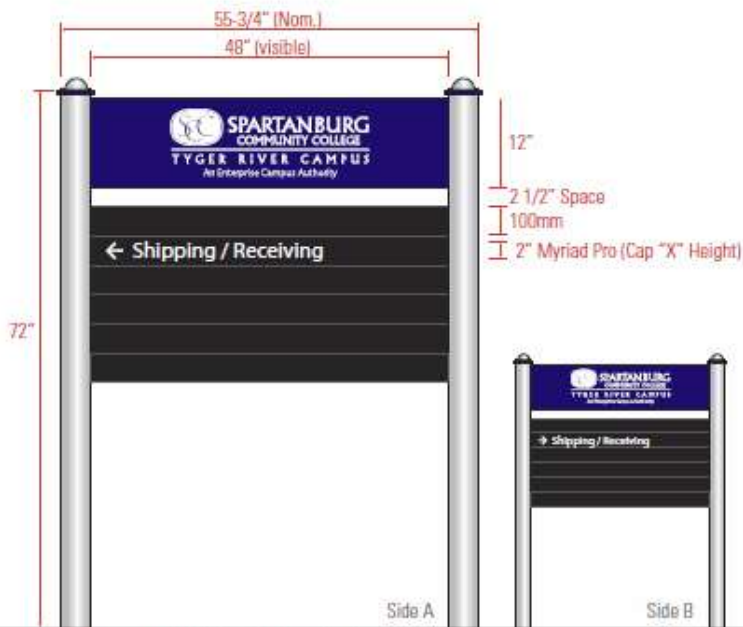
Sign Type A4 / Vehicular Directional Location V.08
